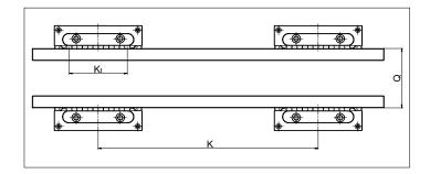
In terms of the spacing K between the recirculating units and the rail spacing Q, the following ratios are recommended as a guideline:
